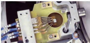
Die is fully tested in the proprietary test nest with the true Kelvin connections to enable measurements at high current
