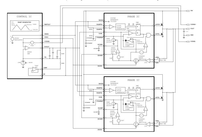
Figure 3 – IR3082PbF PWM Block Diagram
