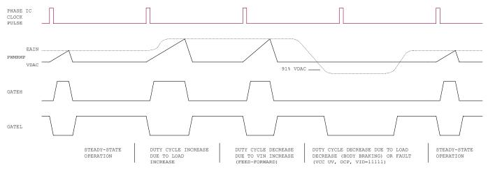
Figure 5 – PWM Operating Waveforms
