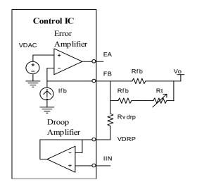
Figure 9 - Temperature compensation of inductor DCR
