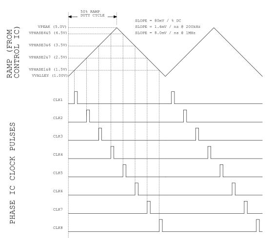
Figure 4 – 8 Phase Oscillator Waveforms
