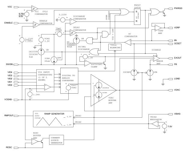
Figure 7 – IR3082PbF Block Diagram
