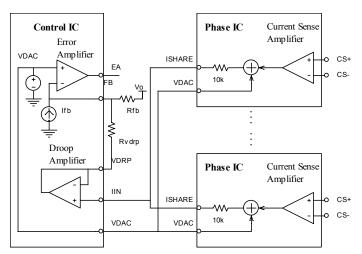
Figure 8 - Adaptive voltage positioning
