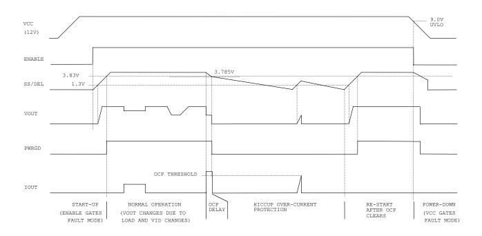
Figure 11 – Operating Waveforms
