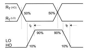
Figure 2. Switching Time Waveform Definitions
