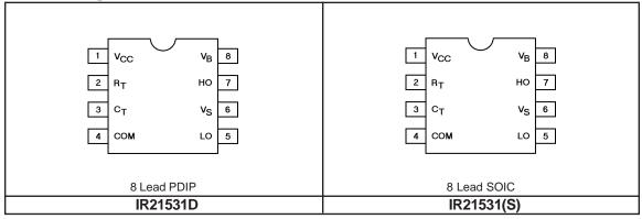
NOTE: The IR21531D is offered in 8 lead PDIP only.
