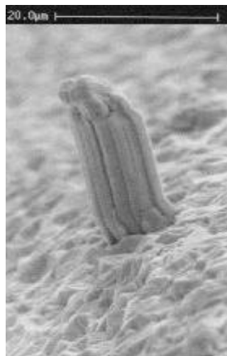
Figure 4. Example of a tin whisker grown on a pure tin plated surface
