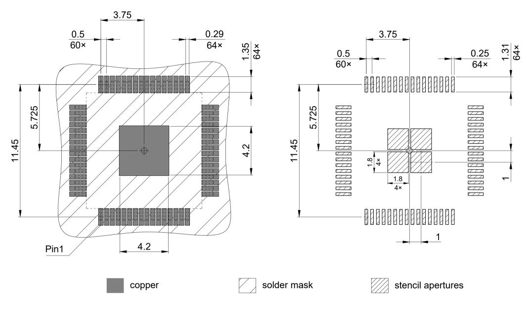
All pads are non-solder mask defined All dimensions are in units mm
