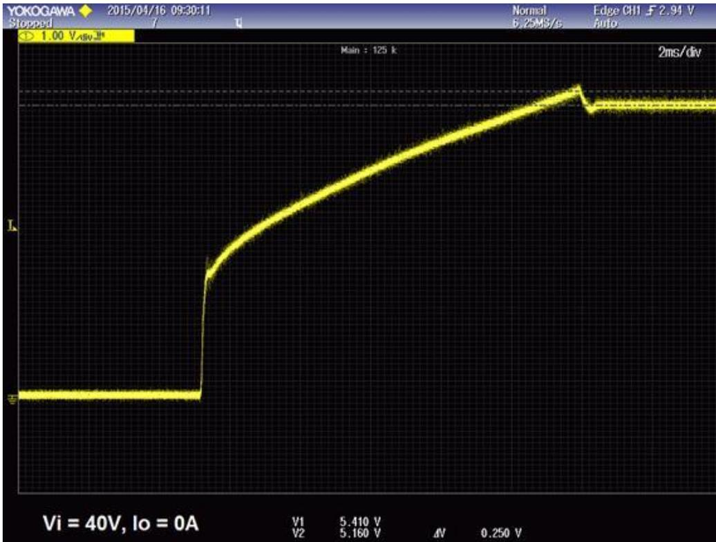
Fig. Fig. (12) Turn ON output voltage transient at no load and maximum line input voltage of 40 VDC at 25 °C
