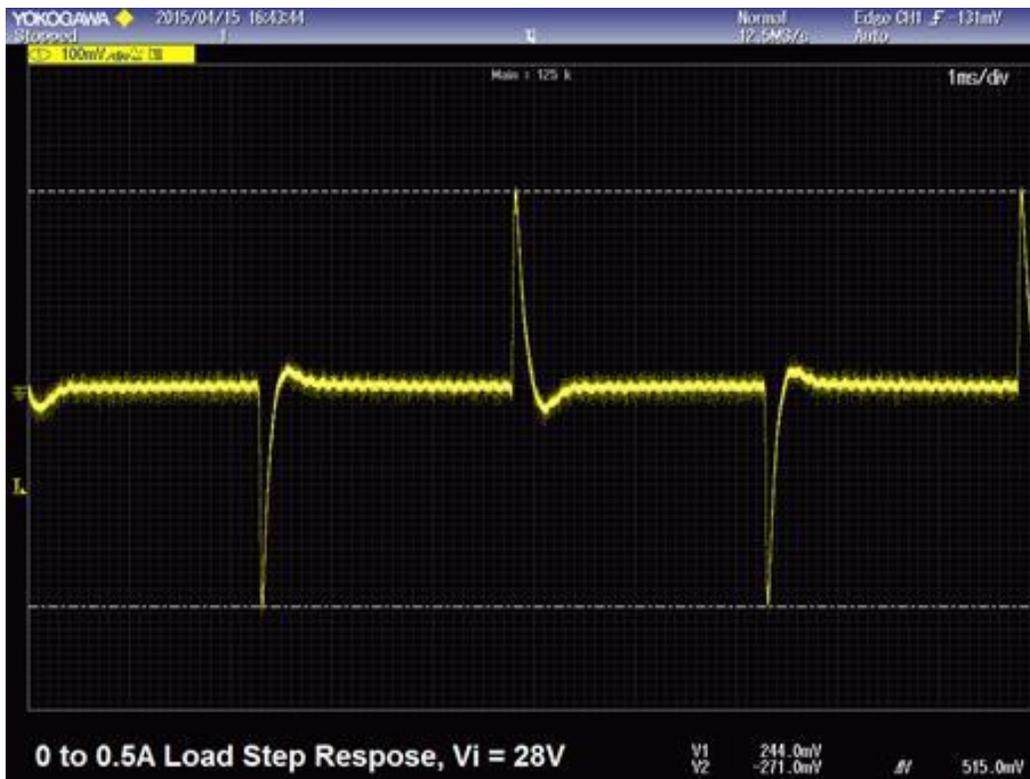
Fig. (10) Dynamic Response of output when input=28VDC and output load is switched from 0.0 to 50% at 25 °C
