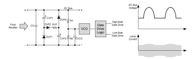
Fig. 3, Passive PFC control circuit.
