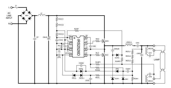
Fig. 5, 26W electronic ballast circuit schematic.
