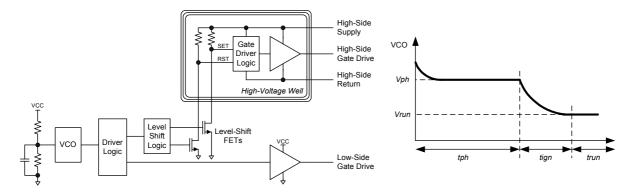
Fig. 2, Voltage-controlled oscillator (VCO) and half-bridge control circuit.
