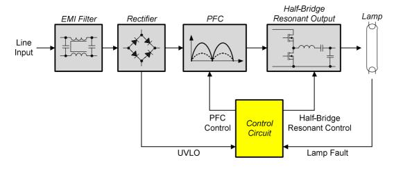
Fig. 1, Electronic ballast block diagram.
