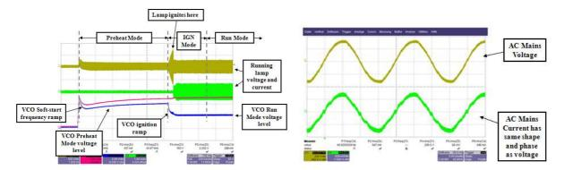
Fig. 8, 2x54W/T5 ballast waveforms. Normal preheat, ignition, run output waveforms (left waveforms) and AC mains input voltage and current (right waveforms).
