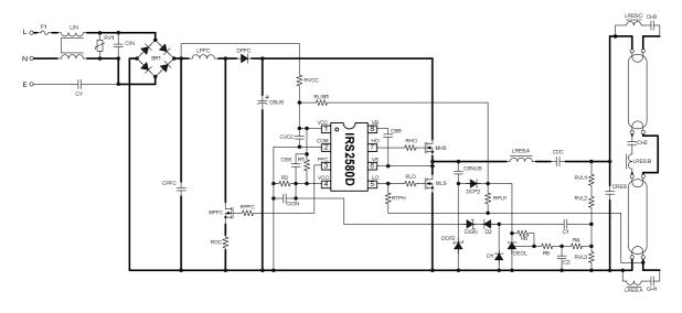
Fig. 6, 2x54W/T5 electronic ballast circuit schematic.
