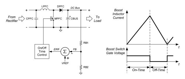
Fig. 4, Boost PFC control circuit.
