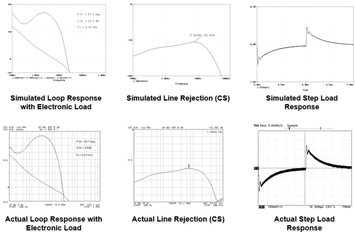
Fig. 2. Simulation example for a hybrid dc-dc converter circuit: simulated vs. actual (measured) results.
