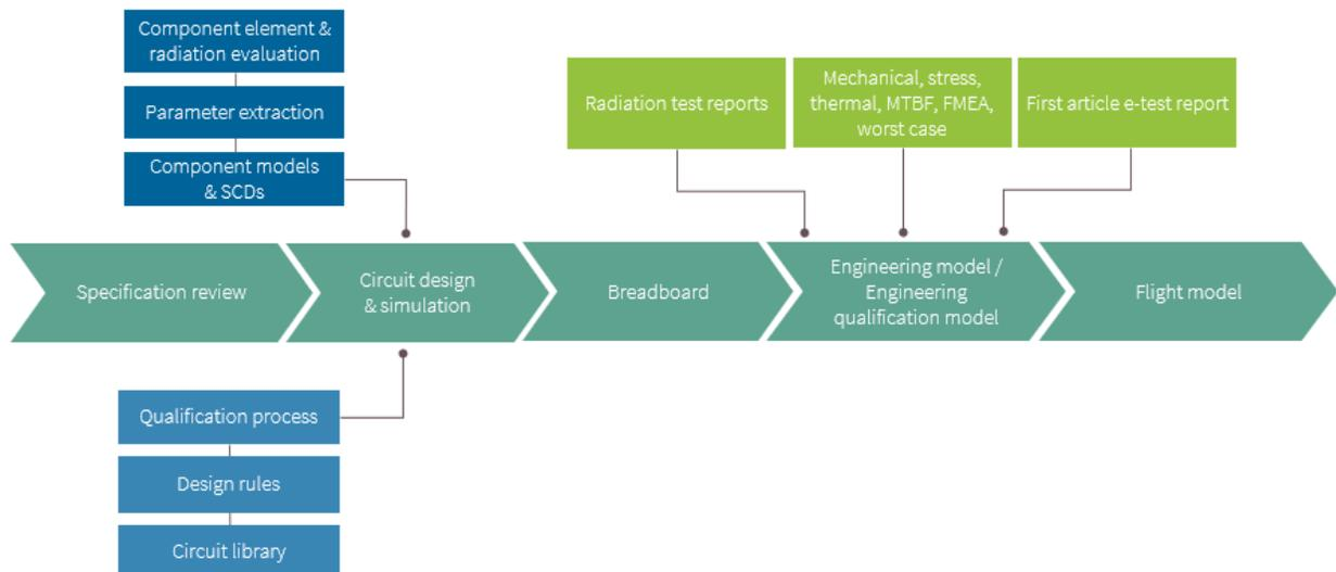
*Fig. 1. Design flow to production for IR HiRel's Class K hybrid dc-dc converters.*
