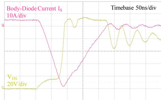
Fig. 6a Typical reverse-recovery waveform from device A1
