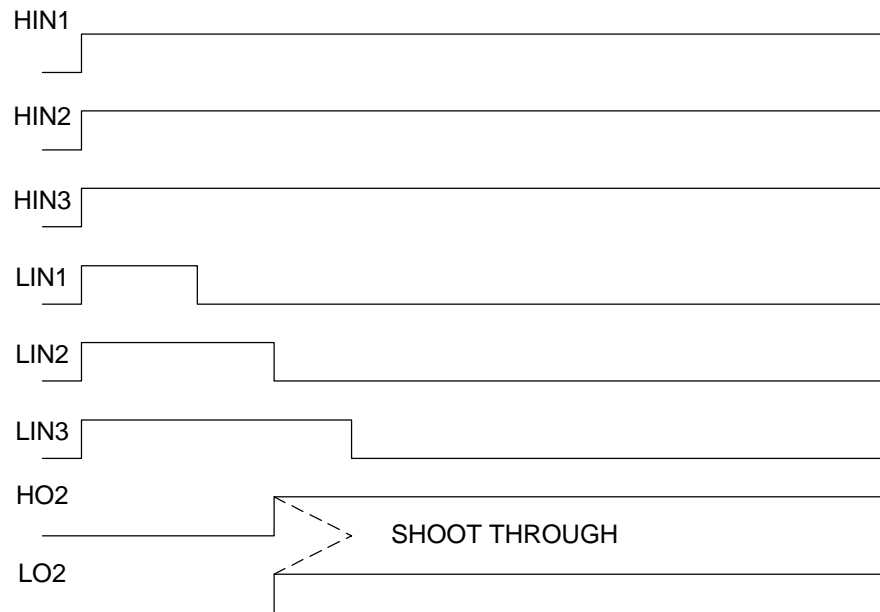
Figure 1: Power up sequence of Bootstrap Capacitor Charging
