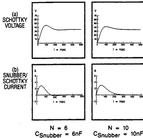
Figure 51. Waveforms of (a) commutating voltage across Schottky and (b) combined current in snubber and self-capacitance of Schottky, for different values of snubber capacitance. ( $= N \times$  Schottky Capacitance).
