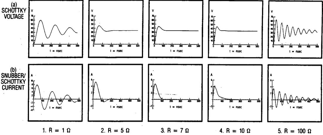
**Figure 49.** Waveforms of (a) commutating voltage across Schottky and (b) combined current in snubber and self-capacitance of Schottky, for various values of snubber resistance.  $N = C_{\text{Snubber}}/C_{\text{Schottky}} = 6$ .
