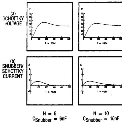
Figure 52. Waveforms of (a) commutating voltage across Schottky and (b) combined current in snubber and self-capacitance of Schottky, for different values of snubber capacitance. ( $= N \times$  Schottky Capacitance).
