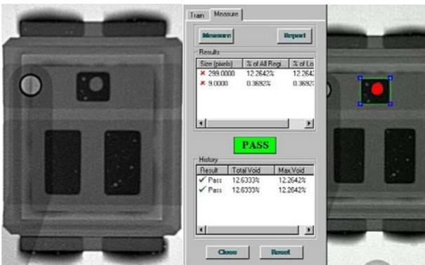
Figure 12 Voids on the gate contact
