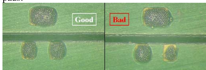
Figure 7 Images showing a good solder print and a bad solder print
