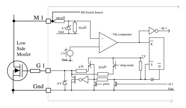
The core of this Shoot-Through circuitry is composed of a RS Flip-Flop and a voltage comparator. This configuration memorizes the request of the HS turn-on and the latter resets the memory when it is fully OFF ([M1-Gnd] < 2V). One can notice that the low side driver features a low consumption "Sleep Mode Pull-up" for the quiescent ON state. Although the PWM signal is sent to both LS MOSFETs at the same time, the leg with the IN input at 0V is the only one that cycles its LS MOSFET.
