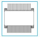
25 Amp. Push-Pull 3-Phase Brushless **DC Motor Controller/Driver Module** in a Power Flatpack
