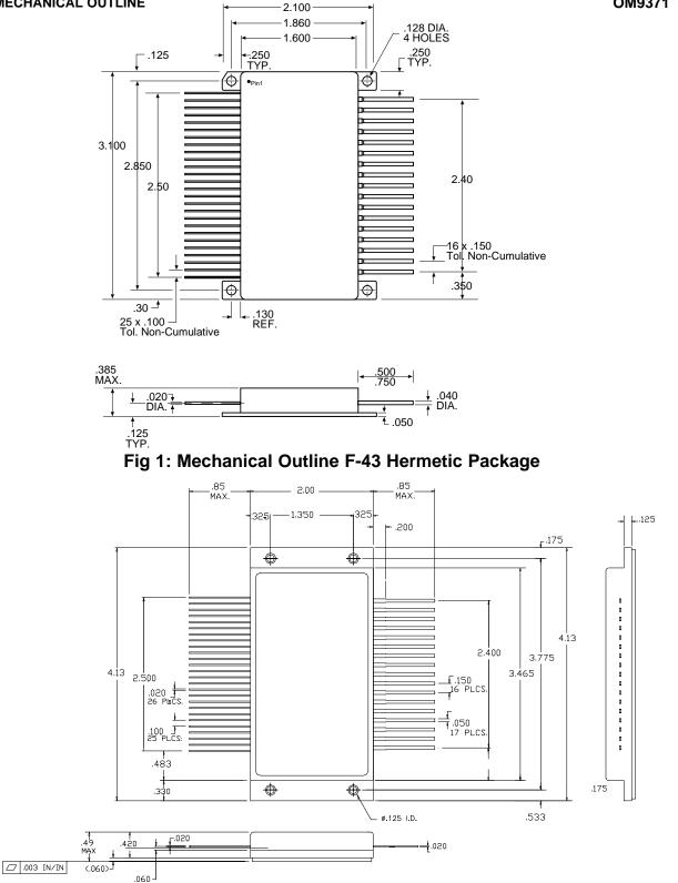
Fig 2: Mechanical Outline MP3-43L Plastic Ring Frame Package
