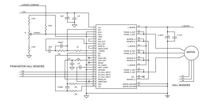
Fig 5: Implementation of a Current-Mode Controller
