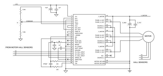
Fig 4: Implementation of a Voltage-Mode Controller
