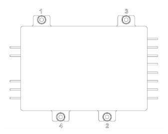
5. Tighten the screws with an appropriate torque driver. Torque the screws up to 6 in lb in the sequence shown above
