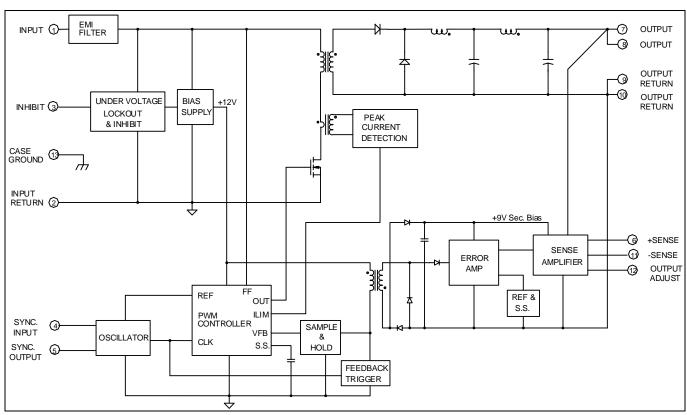
Figure 1 Block Diagram - Single Output
