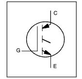
600 V  $I_{C(nom)} = 24A$   $V_{CE(on)} \text{ typ.} = 1.60 \text{ W}$   $I_{C(nom)} \text{ @ } 25^{\circ}\text{C}$ Motor Control IGBT
