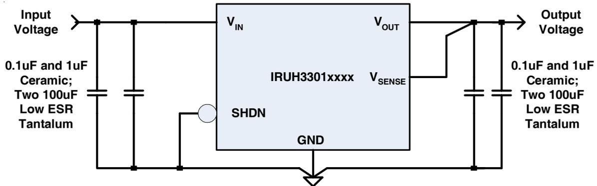
**Fig. 1.** Typical Regulator Circuit; Note the SHDN Pin is hardwired in the “ON” position.
