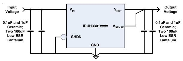
**Fig. 1.** Typical Regulator Circuit; Note the SHDN Pin is hardwired in the "ON" position. The  $V_{SENSE}$  Pin is connected as noted in the "General Layout Rules" section.
