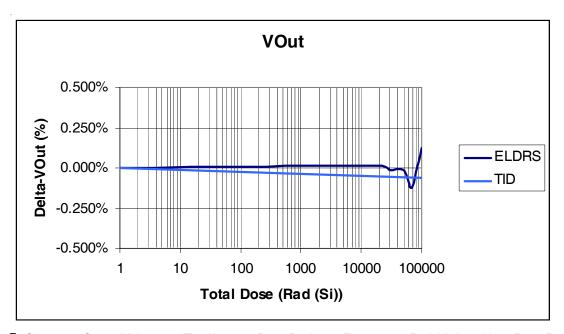
Fig. 5. Change in Output Voltage vs. Total Ionizing Dose Radiation Exposure at Both High and Low Dose Rates
