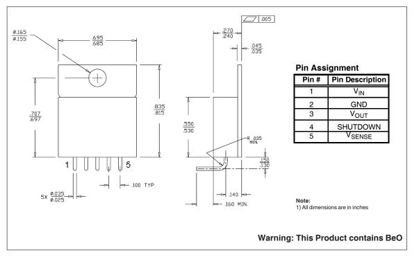
Fig 9. Case Outline and Dimensions - MO-078AA (Lead Trimmed)
