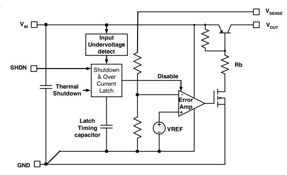
Fig. 3. Simplified Schematic Circuit
