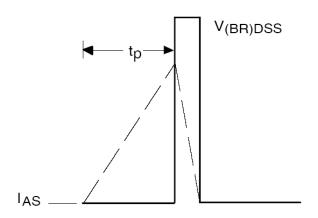
Fig 12b. Unclamped Inductive Wave-
