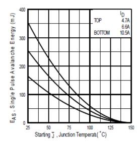
Fig 10. Maximum Avalanche Energy Vs. Drain Current
