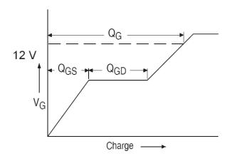
Fig 13a. Gate Charge Waveform
