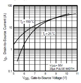
Fig 3. Typical Transfer Characteristics
