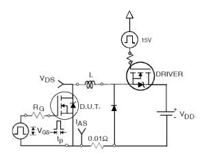
Fig 12a. Unclamped Inductive Test Circuit
