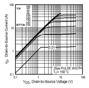
Fig 2. Typical Output Characteristics
