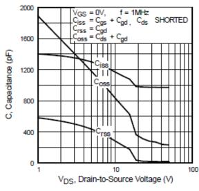
Fig 5. Typical Capacitance Vs. Drain-to-Source Voltage
