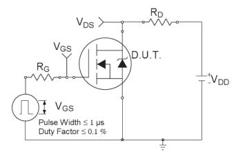
Fig 14a. Switching Time Test Circuit
