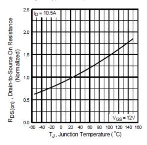
Fig 4. Normalized On-Resistance Vs. Temperature
