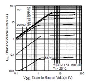
Fig 1. Typical Output Characteristics
