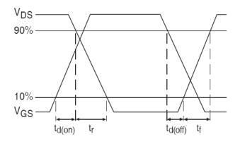
Fig 14b. Switching Time Waveforms
