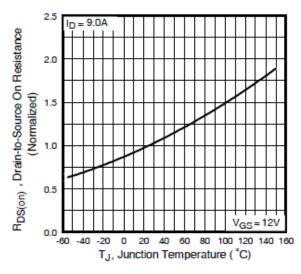
**Fig 4.** Normalized On-Resistance Vs. Temperature
