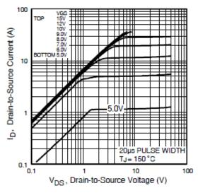
Fig 2. Typical Output Characteristics
