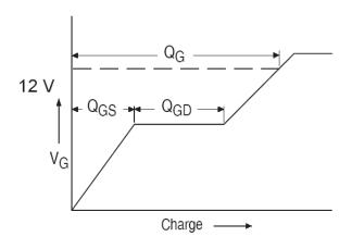
Fig 13a. Gate Charge Waveform
