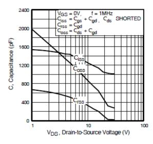
**Fig 5.** Typical Capacitance Vs. Drain-to-Source Voltage
