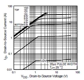
Fig 1. Typical Output Characteristics
