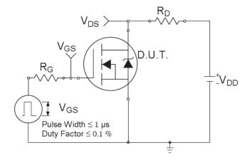
Fig 14a. Switching Time Test Circuit
