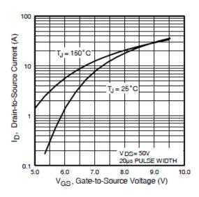
Fig 3. Typical Transfer Characteristics
