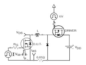
Fig 12a. Unclamped Inductive Test Circuit
