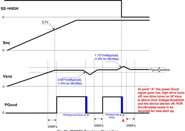
Fig.9b IR3859 Tracking Operation
