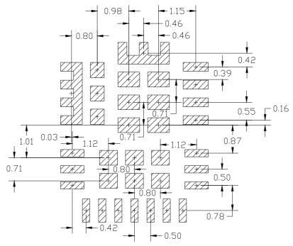
Stencil pad spacing (all dimensions in mm)
