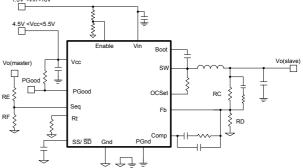
Fig. 8b. Application Circuit for Simultaneous Sequencing
