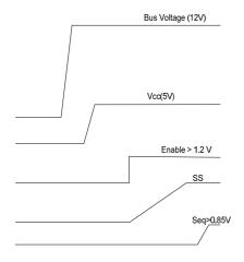
Fig. 3c. Recommended startup sequence, Sequenced operation
