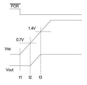
Fig. 6. Theoretical operation waveforms during soft-start
