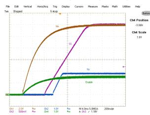
Fig. 18: Start up at 9A Load  $Ch_1:V_{in}, Ch_2:V_{out}, Ch_3:V_{ss}, Ch_4:Enable$
