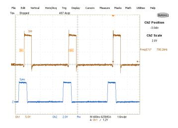
Fig. 26: Synchronization to 700kHz external clock signal at 9A load Ch<sub>1</sub>: SW (Switch Node) Ch<sub>2</sub>:Sync
