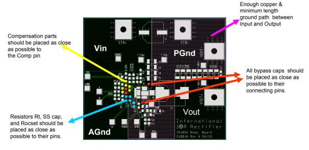
Fig. 28a. IRDC3859 demoboard layout considerations – Top Layer
