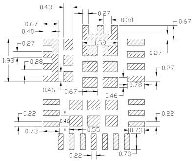
Stencil pad sizing (all dimensions in mm)
