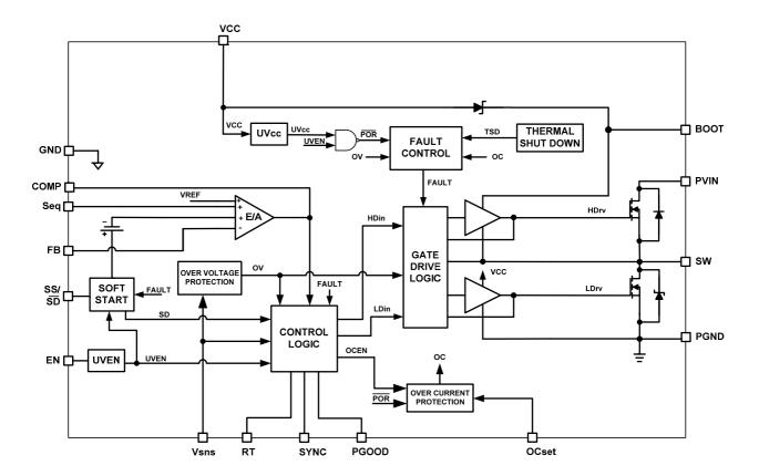
Fig. 2. Simplified block diagram of the IR3859
