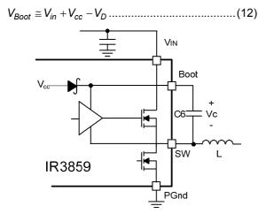
Fig. 13. Bootstrap circuit to generate Vc voltage
