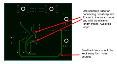
Fig. 28d. IRDC3859 demoboard layout considerations - Mid Layer 2
