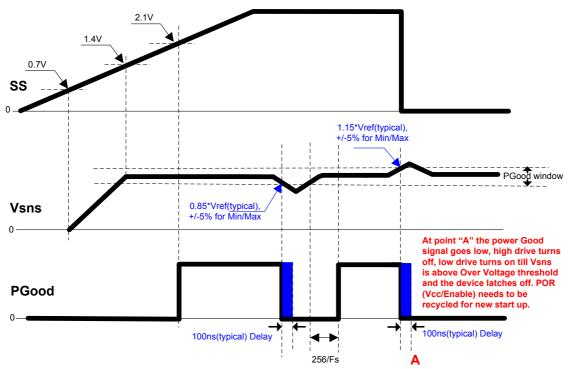
Fig.9a IR3859 Non-Tracking Operation (Seq=Vcc)
