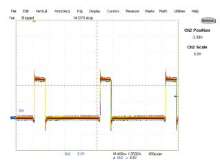
Fig. 22: Inductor node at 9A load Ch<sub>2</sub>: Switch Node
