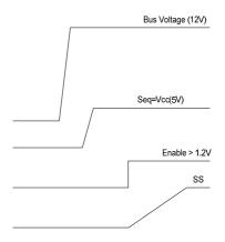
Fig. 3b. Recommended startup sequence, Non-Sequenced operation
