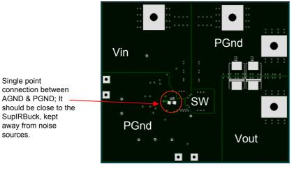
Fig. 28b. IRDC3859 demoboard layout considerations – Bottom Layer
