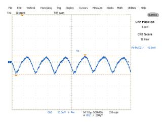
Fig. 21: Output Voltage Ripple, 9A load Ch<sub>2</sub>: V<sub>out</sub>
