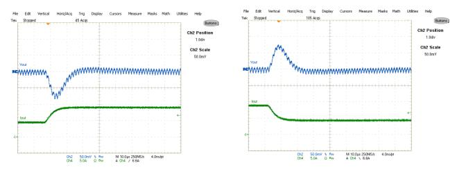
Fig. 24: Transient Response, 4.5A to 9A step  $2.5A/\mu s$   $Ch_2:V_{out}, Ch_4:I_{out}$
