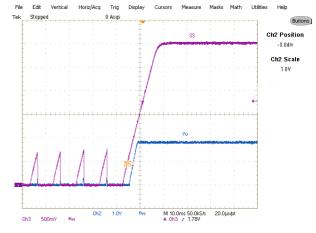
Fig. 23: Short (Hiccup) Recovery Ch<sub>2</sub>:V<sub>out</sub>, Ch<sub>3</sub>:V<sub>ss</sub>
