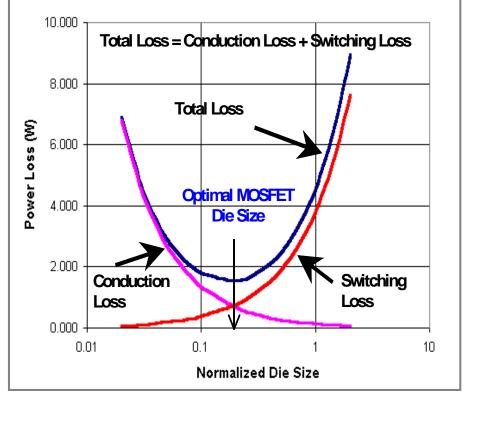
Optimal MOSFET die size  $\Rightarrow$  Optimal MOSFET Parameters
