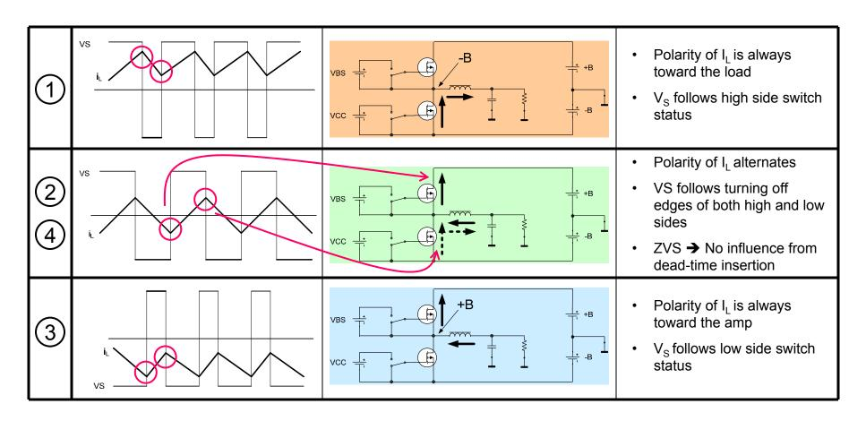
Note: Dead-time insertion reduces volt-second of  $V_s$ . Dead-time inserted in the rising edge of the high side affects the operating region 1. Dead-time inserted in the rising edge of the low side affects the operating region 3. As a result, output voltage gets lower than it should be, causing non-linearity in the output stage.
