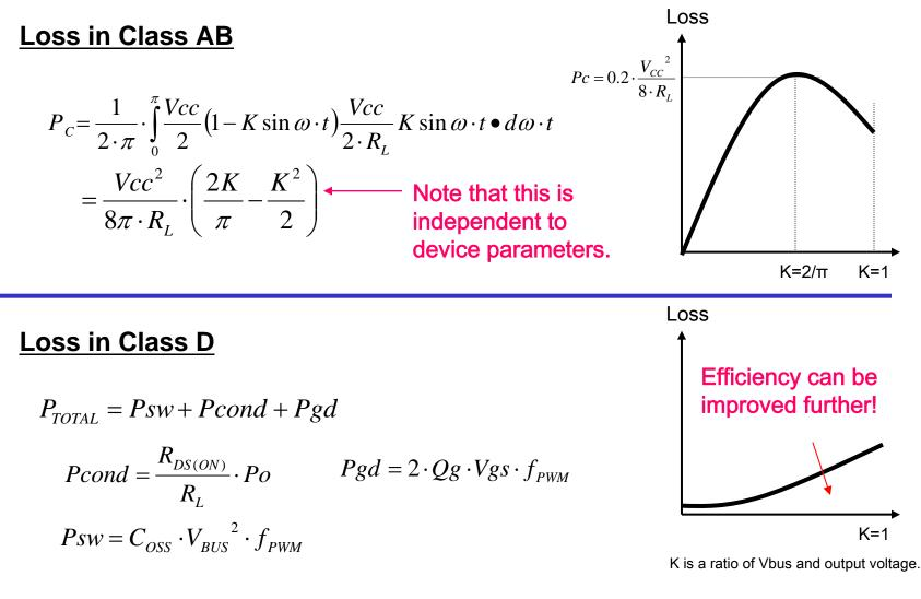
To learn more about power losses in Class D, refer to AN-1070 Class D Amplifier Performance Relationship to MOSFET Parameters.
