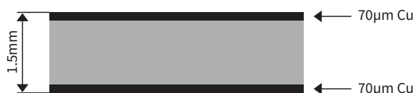
Cross section JEDEC 1s0p board
