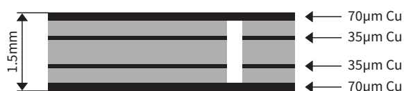
Cross section JEDEC 2s2p board
