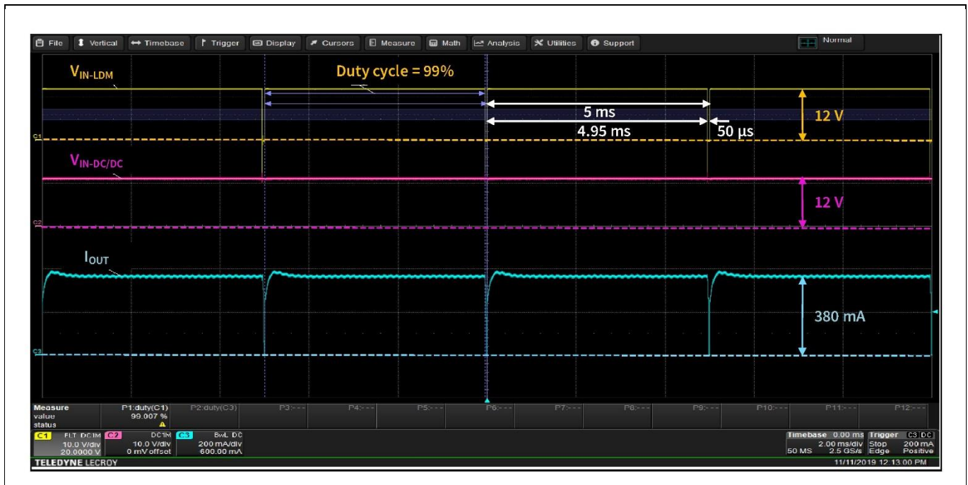
Figure 6 Measurement on real case with TLD5098 with 200 Hz rectangular waveform with 99% duty cycle
