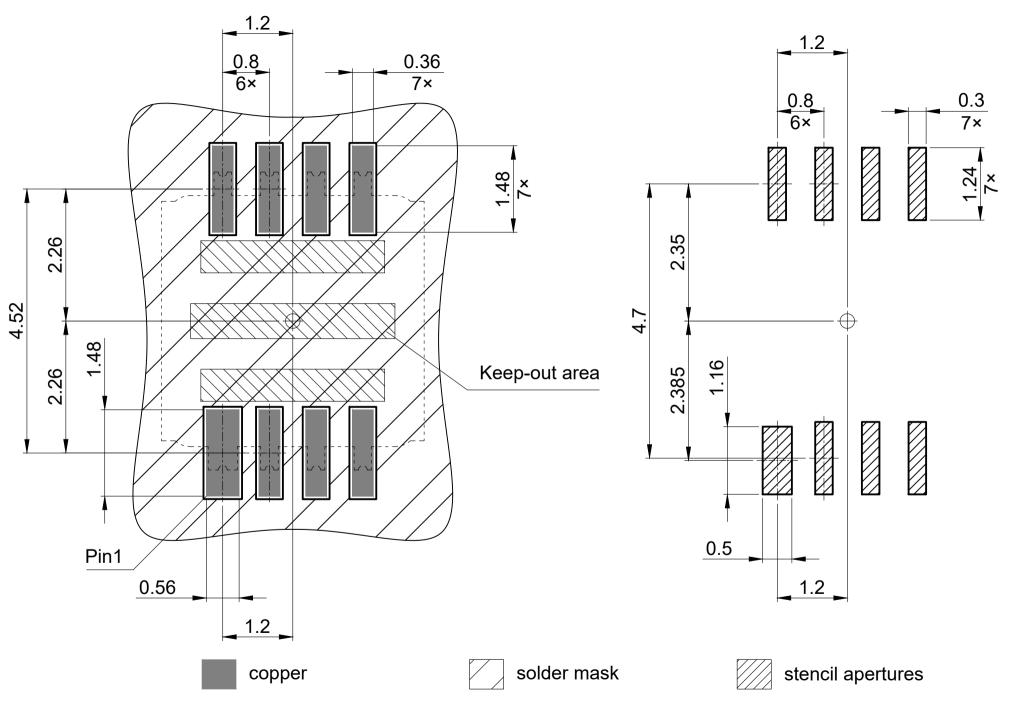
Based on stencil thickness 0.13 mm All dimensions are in units mm
