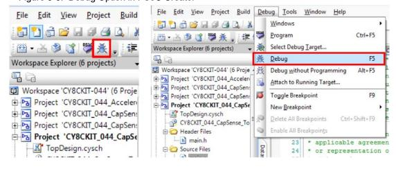
2. When PSoC Creator enters the Debug mode, use the buttons on the toolbar or keyboard short-cuts to debug your project.
