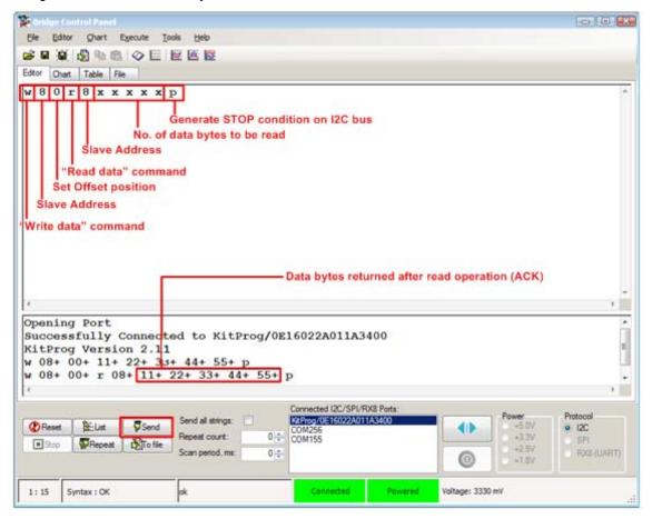
**Note:** You can add additional lines of commands by pressing **[Ctrl] [Enter]**. To execute any line, click on that line and press **[Enter]** or click the **Send** button.
