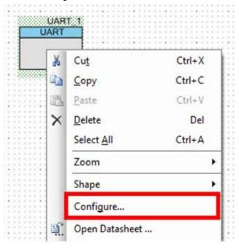
3. Configure the UART Component as shown in Figure 5-4, Figure 5-5 and Figure 5-6, and then click **OK**.
