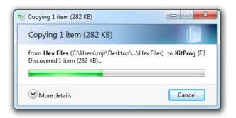
4. The Status LED on the kit blinks during the programming operation. The Status LED continues to blink for 2 seconds after the programming operation and the KitProg Drive automatically removes the copied file from the drive. Press **F5** in the file explorer to refresh the contents of the drive. This will display only the STATUS.TXT file in the KitProg Drive.
