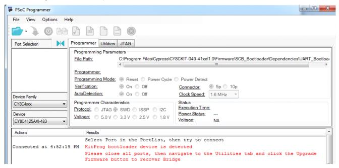
4. Switch to the **Utilities** tab in PSoC Programmer and click the **Upgrade Firmware** button, as shown in Figure 8-2. Unplug all other PSoC programmers (such as MiniProg3 and DVKProg) from the PC prior to clicking the **Upgrade Firmware** button.
