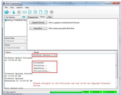
6. The factory program is now successfully restored on the PSoC 5LP. It can be used as the programmer/debugger for the PSoC 4200M device.
