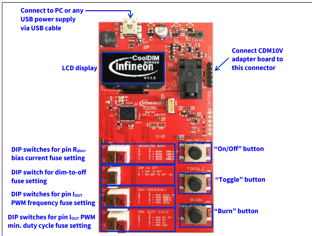
Figure 22 CDM10V programming board and hardware connection set-up for CDM10V configuration
